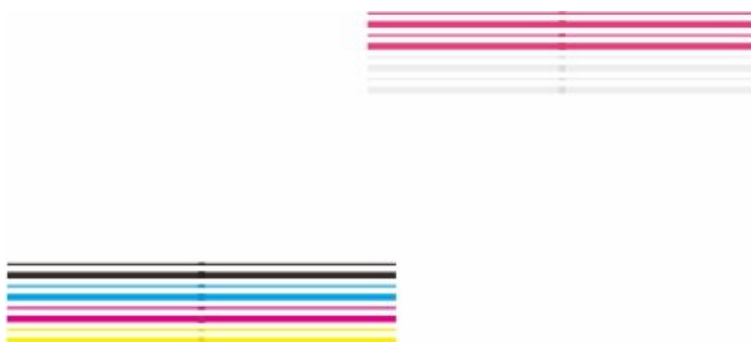
图4.3.3 Correct vertical calibration
