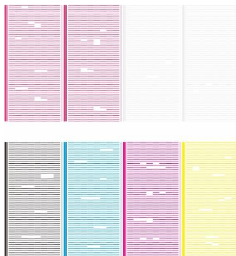
图4.3.2 Incomplete test strip
