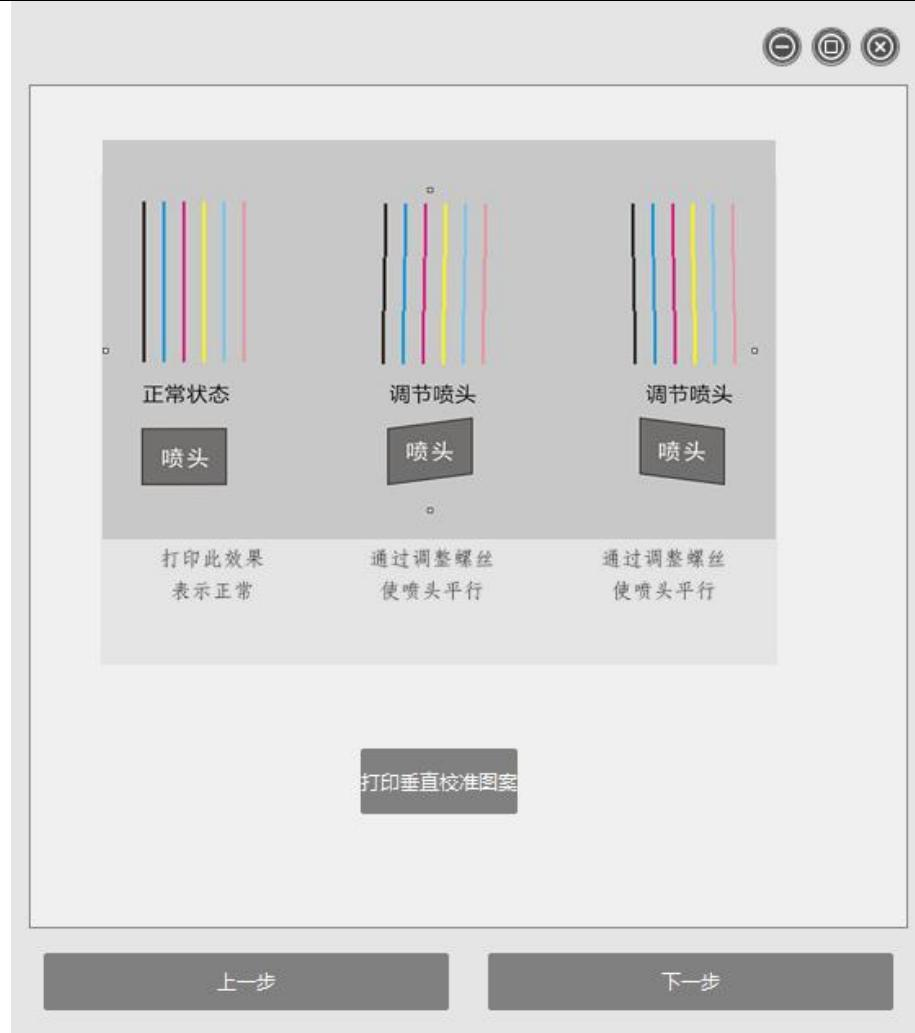
**Click “Print vertical and calibration pattern” . Adjust the white, color and varnish head and then click Next. The software will enter the main calibration interface and choose Horizontal spacing calibration for heads automatically.**
