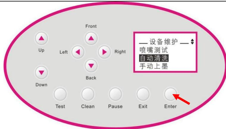
Then click “Automatic cleaning”, click on the “Enter” button, and the machine will clean the printhead automatically.
