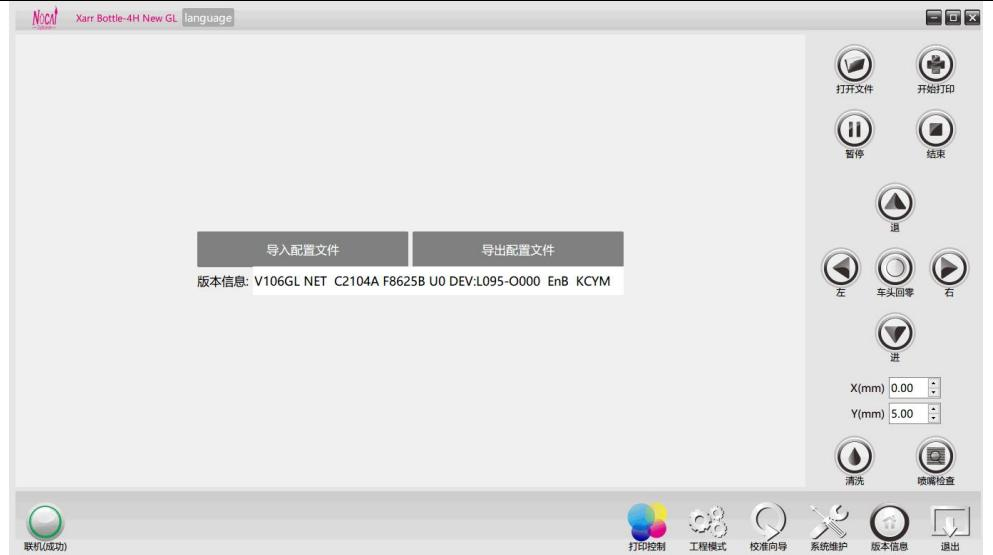
**Export configure file:** Export the parameter settings in the on-line software to a file with a pfg suffix format for backup.
