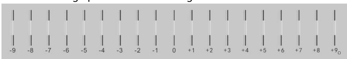
Look at the graphic to see how well the black and white lines coincide. For example, the "+3" black and white lines are the best to coincide, and the current horizontal spacing coefficient is increased by 3; If the "-3" black and white lines coincide best, the current horizontal spacing coefficient will be reduced by 3. Debug it several times until the black and white lines corresponding to the number "0" have the best degree of coincidence, which is a straight line.
