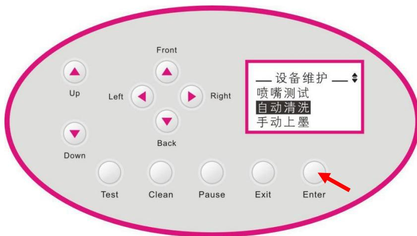
Refer to the following **sampling operation** as the following, place a bottle on the platform and click on the “Nozzle test” to print the test strip, if there is a lack of color or ink-suspension phenomenon, please continue to clean the printhead until the test strip are complete, ink installation is completed.
