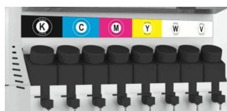
In order to prevent the ink from leaking out and contaminating the shell sheet metal when adding the ink, protective measures need to be taken. The bottle mouth can be wrapped with paper.
