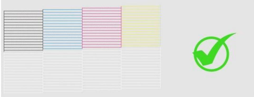
If the test strip breaks, you need to "Clean automatically"
