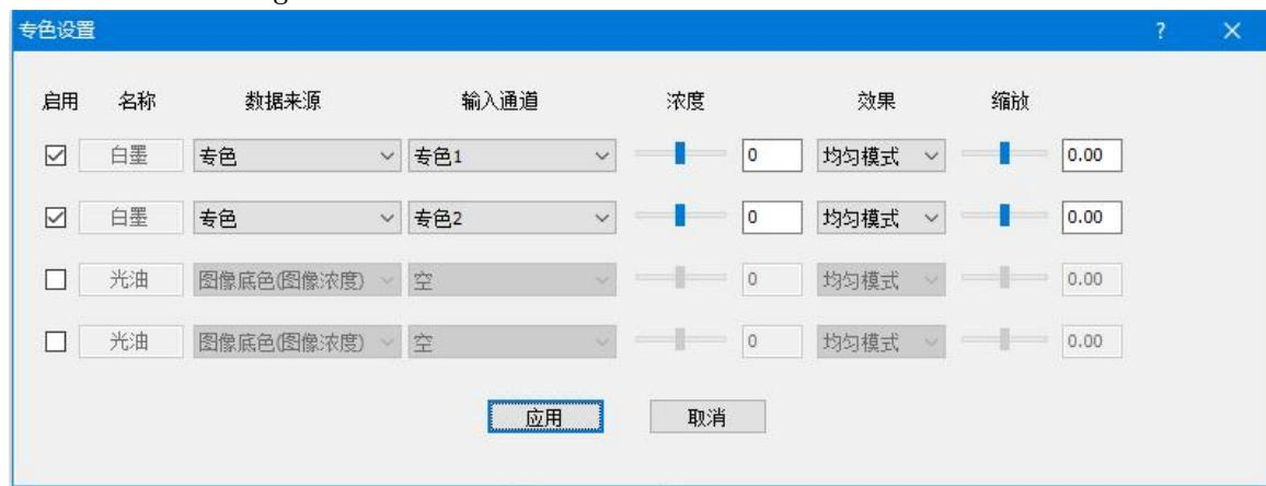
**Start:** Checking the box starts printing in the corresponding spot color, while leaving it unchecked does not start spot color printing.
