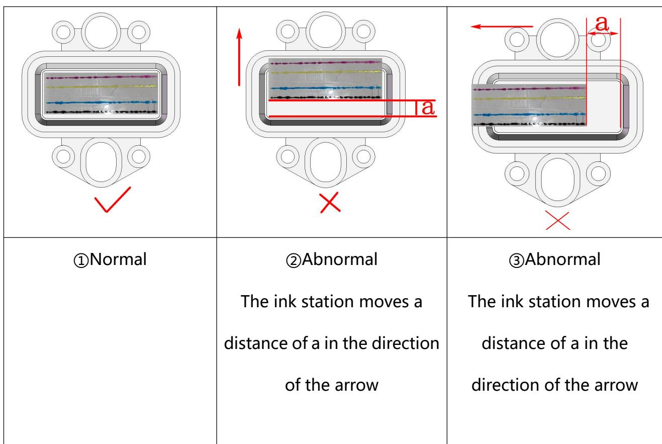
As shown in the figure above, ① is in a normal state, and the flash spray strip is in the center state above the cap top. ②③ In these two typical abnormal problems, the printhead and the cap top are not aligned and sealed, which make it unable to pump ink and the test strip cannot be adjusted normally.
