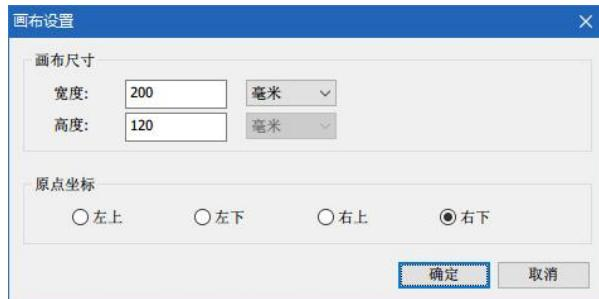
The unit: millimeters; the width: 200; the height: 120; for the original coordinate: right at the bottom. Click OK.
