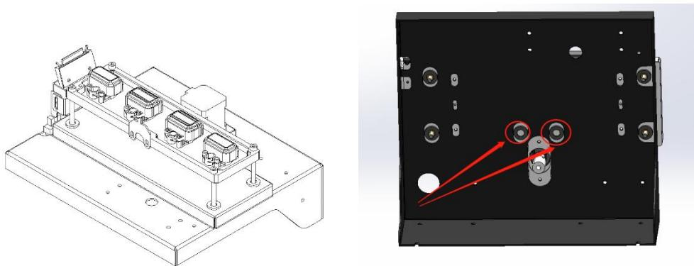
As shown in the figure above, loosen the fixing screws of the ink station (2 arrows) properly, and the cap top can be moved in the direction of the arrow (front and back) as a whole, and after the adjustment is completed, the screws can be tightened.
