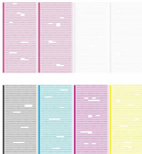
图4.3.2 Incomplete test strip
